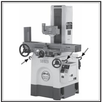
Figure 7. Lifting hooks (3 of 4 shown).
